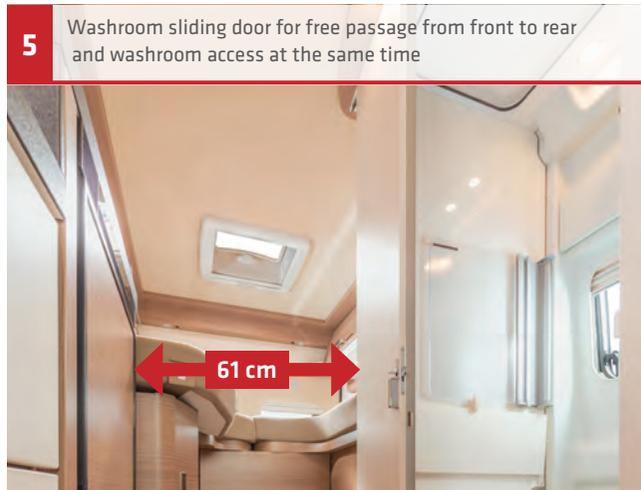
**5** Washroom sliding door for free passage from front to rear and washroom access at the same time
