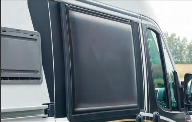
Malibu premium windows with surrounding frames and double sealing system for protection from rain and splash water, additional break-in protection and less driving noise (not with rear windows and porthole windows)
